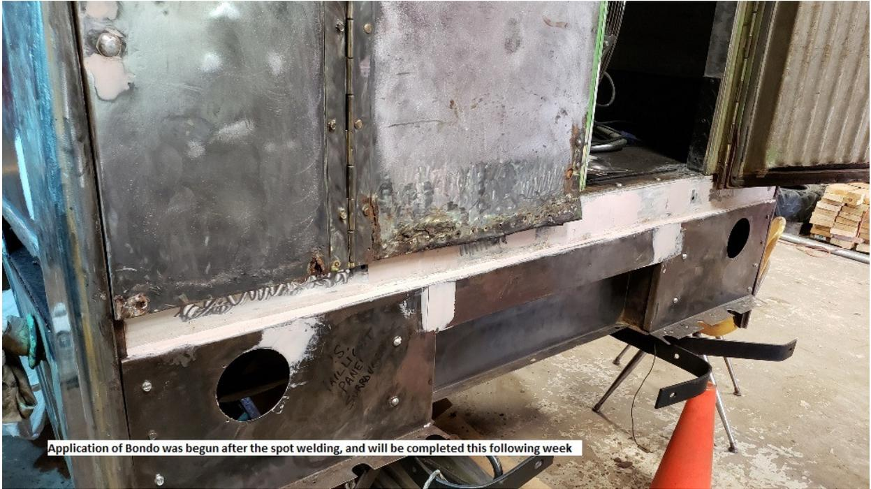
Application of Bondo was begun after the spot welding, and will be completed this following week
