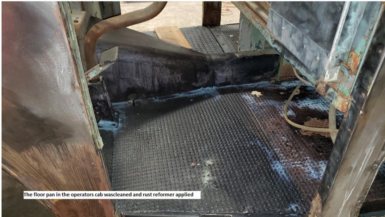
The floor pan in the operators cab was cleaned and rust reformer applied
